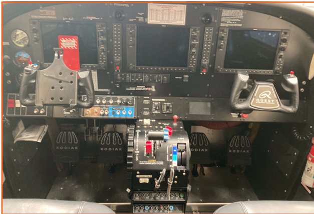
Garmin G1000 Integrated Avionics Suite
